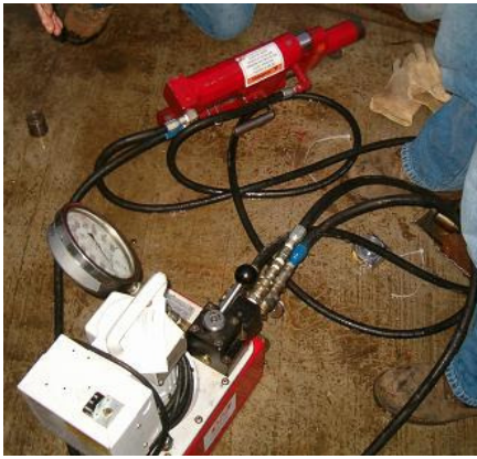
a) Mono-strand jack and hydraulic pump
