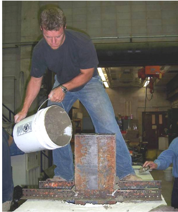
Figure 22. Concrete being placed in the CMP around the H-pile.
