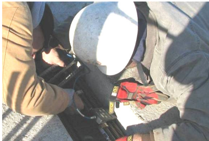
Figure 139. Calibration of one of the vibrating wire gages, November 21.
